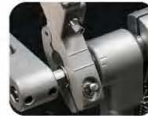
BEATER STROKE ADJUSTMENT A choice of 2 positions for Finesse or Power. Simply loosen the clamshell to change position. US PAT. # 7379540
